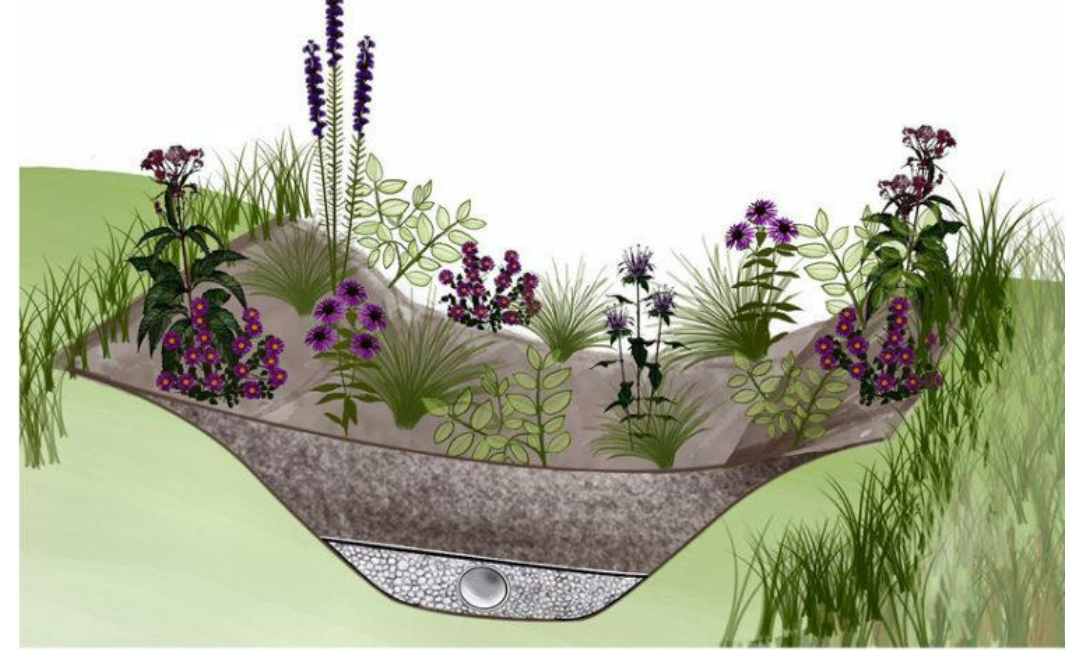
Section drawing of a rain garden
